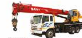
SPC250 Maximum Load Capacity: 25t Telescopic Boom: 4 Sections, 10.22-31.5m
